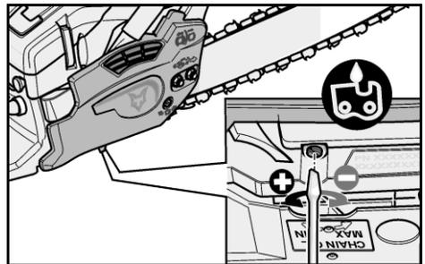
The setting screw for the oil volume is on the underside of the chainsaw.
